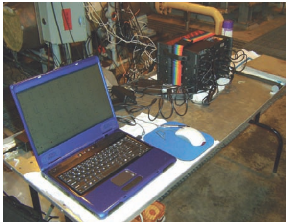
The ZonicBook/618E with expansion modules and a laptop computer collect vibration data during start up and full load to develop a 3D operating deflection model or ODS
