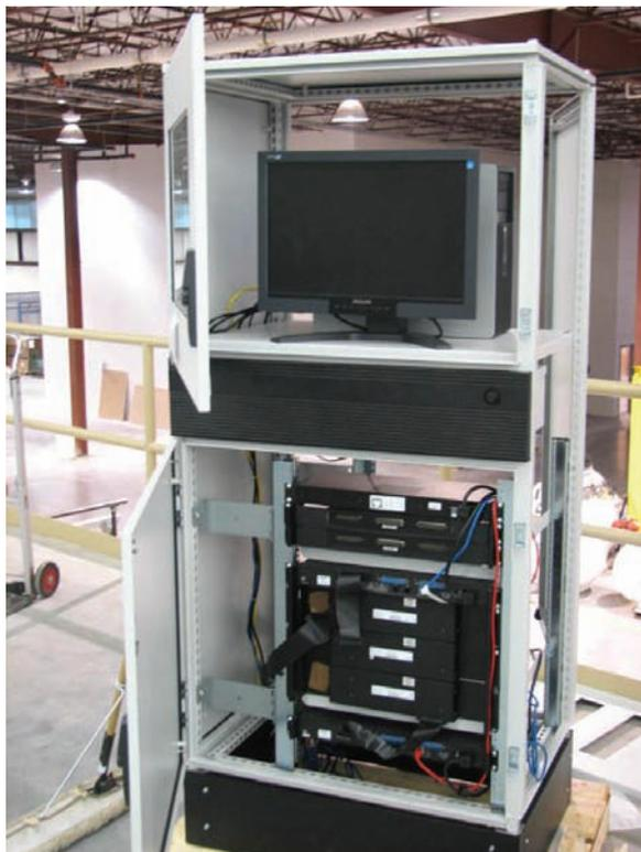
*The data acquisition system is housed in a computer equipment rack. The IOtech DaqScan units are located in the bottom section, while the monitor resides in the top. Doors protect the system from factory floor hazards, but a glass window in the top door lets test engineers see the monitor during operation.*
