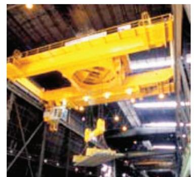
*The Zonicbook/618E was used to take vibration data from each of eight bearing assembly locations and predict wheel assembly failures on NUCOR's billet bay crane.*
