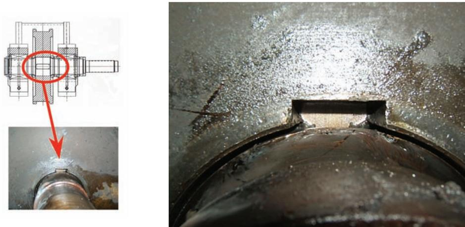
After identifying the wheel assembly with above average vertical amplitudes, the assembly was disassembled, revealing an excessive wheel-to-shaft tolerance. Feeler gauges were used to measure the tolerance which was almost 1/8 of an inch. A visual inspection of the key found that it was loose in the shaft and wheel fit, both vertically and horizontally.
