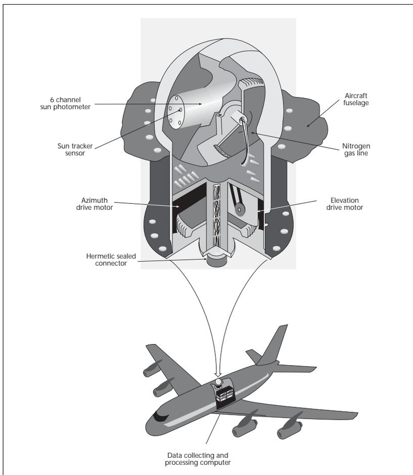
The sun photometer is composed of a solar-tracking system, detector module, temperature control system, nitrogen purge system, mechanical drive train, and data acquisition system
