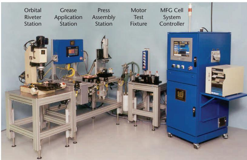
The ATI Systems window motor-module manufacturing cell comprises an orbital riveter, grease application, and press assembly station, as well as a motor test fixture for testing and verification. The IOtech DaqBoard resides in the panel mounted PC within the manufacturing cell system controller. The DaqBoard lets ATI Systems customers improve their reporting, data logging, and analytical capabilities; track warranty related problems; and implement corrective actions during manufacturing.
