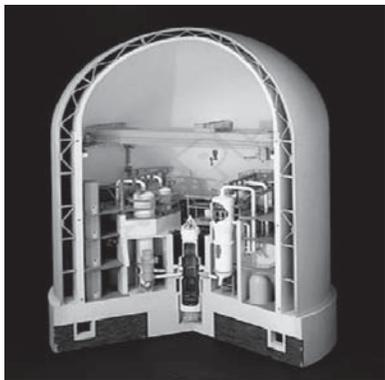
*The first Pressurized Water Reactor built in Britain is based on a US design and produces 1250 MW of carbon-free electricity. The fuel is uranium dioxide, supported in the reactor pressure vessel, which is filled with water under high pressure. Water is pumped through the reactor to carry heat away from the fuel. The hot water passes through a heat exchanger that heats a second supply of water. The secondary water boils, and the resulting steam drive the electric generators.*
