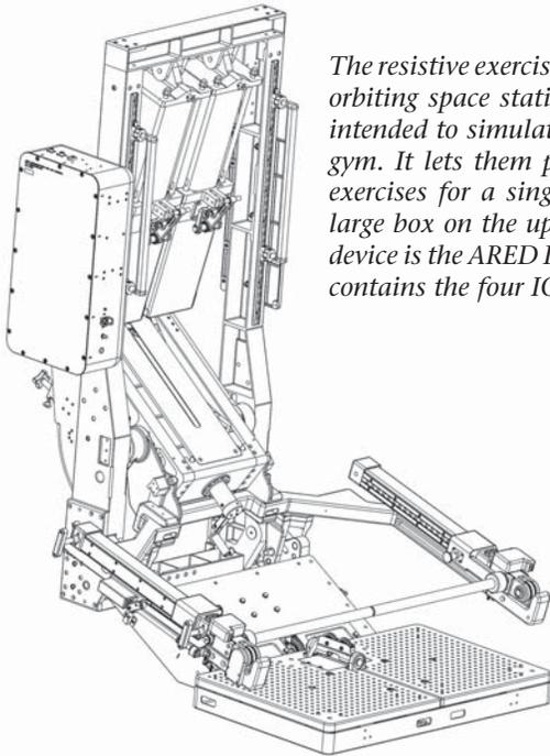
*The resistive exerciser used by astronauts on the orbiting space station is a full body exerciser, intended to simulate free weights, like a home gym. It lets them perform cable and bar-type exercises for a single hand, leg, or limb. The large box on the upper left side of the exercise device is the ARED Instrumentation Box, which contains the four IOtech Personal Daqs.*
