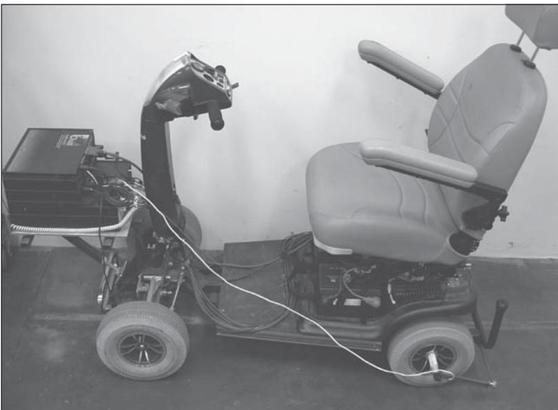
Although Electric Mobility uses stationary fatigue-cycling machines to test mechanical parts for durability with a variety of sensors that can detect catastrophic failures, it also measures mechanical dynamic variables on working prototypes such as acceleration, speed, distance, and rollback, as well as electrical variables including motor/controller temperature, current, and voltage.
