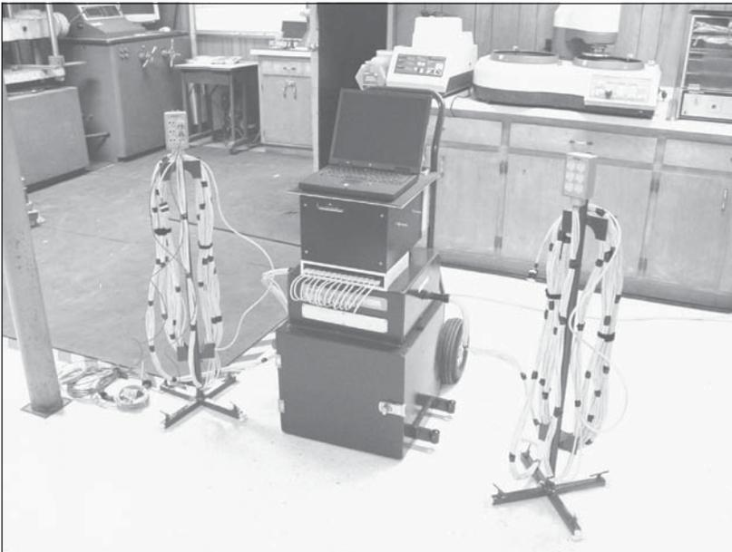
GIW Industries, Grovetown, Georgia, devised a mobile data acquisition system in a small cart, which contains an IOtech **DaqBook** and signal conditioners, a laptop computer, and special thermocouple cables for measuring the temperatures of cast components during various processing steps in manufacturing and development.
