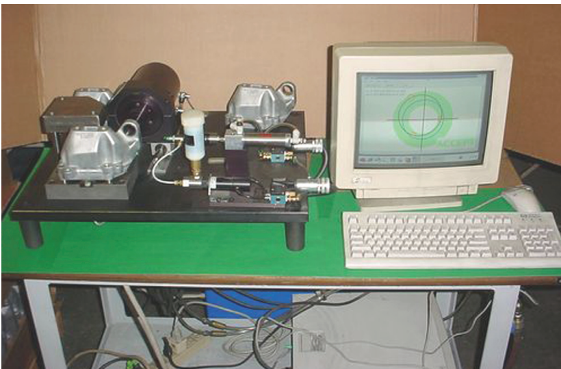
The Skrl Diecasting production line measurement system incorporates an IOtech DaqBoard located in the PCI slot of the desktop computer on the right. The die cast bracket under test is shown on the left side of the platform with the LVDT-based probe measuring the hole size and location. Two air cylinder control valves regulate the speed of the air cylinder that positions the three-pronged probe.
