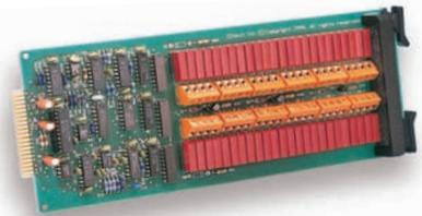
**MTC/24 Thermocouple/Volt Scanning Module.** The MTC/24 provides 24 isolated differential input channels, and per-channel programmability for thermocouple types J, K, T, E, R, S, B, and N, or for  $\pm 10\text{V}$ ,  $\pm 5\text{V}$ ,  $\pm 1\text{V}$ , and  $\pm 100$  mV inputs. Channel-to-channel isolation is 200 VDC peak.
