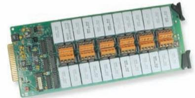
**MHV/24X High-Voltage Scanning Module.** The MHV/24X provides 24 differential voltage-input channels, and per-channel programmability for  $\pm 250\text{V}$ ,  $\pm 25\text{V}$ , and  $\pm 2.5\text{V}$ . Channel-to-channel isolation is 500 VDC peak.
