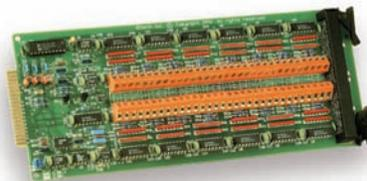
**TempRTD/16B RTD Scanning Module.** The TempRTD/16B scanning module supports 16 channels of 3- or 4-wire RTDs. Measurements may be designated in units of  $^{\circ}\text{C}$ ,  $^{\circ}\text{F}$ ,  $^{\circ}\text{K}$ , or  $^{\circ}\text{R}$ .
