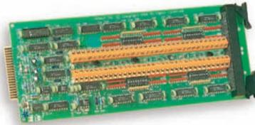
**TempTC/32B Thermocouple Scanning Module.** The TempTC/32B thermocouple scanning module contains 32 differential input channels, each of which may be configured for thermocouple types J, K, T, E, R, S, B, and N, or for a  $\pm 100$  mV input. Measurements may be designated in units of  $^{\circ}\text{C}$ ,  $^{\circ}\text{F}$ ,  $^{\circ}\text{K}$ ,  $^{\circ}\text{R}$ , or volts.
