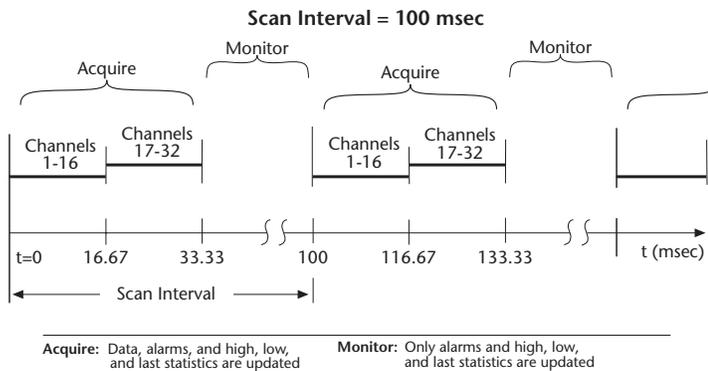
The TempScan/1100's programmable scan interval controls the time between successive channel scans, as illustrated in the above example for a 32-channel system
