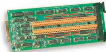
**TempV/32B Voltage Scanning Module.** The TempV/32B scanning module contains 32 differential input channels and is capable of measuring voltage with programmable ranges of  $\pm 10\text{V}$ ,  $\pm 5\text{V}$ ,  $\pm 1\text{V}$ , and  $\pm 100$  mV.
