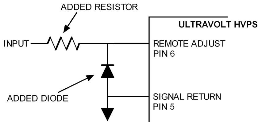
The added shunt diode is a standard low forward voltage drop diode (for example, the low-cost 1N4001), and the added resistor is chosen to limit the current (for example, a 1kΩ resistor would limit a -5V input remote adjust input to 5mA).
