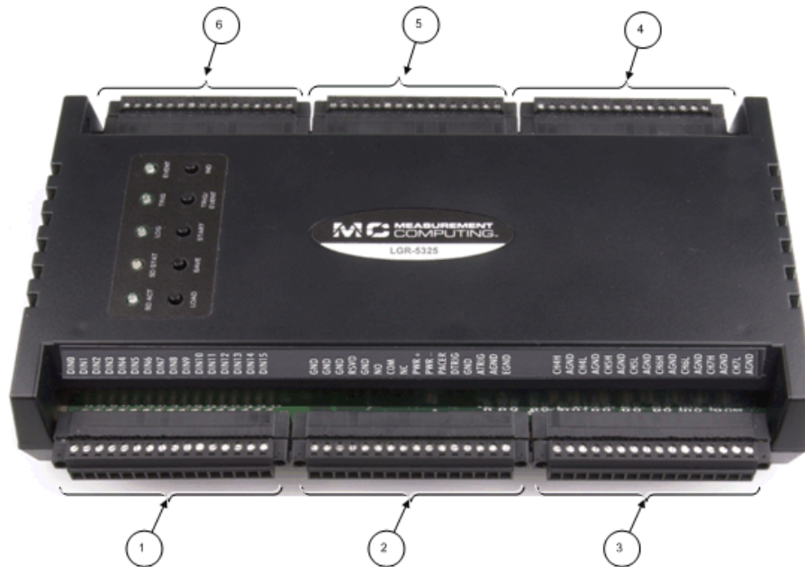
Figure 6. LGR-5325 front screw terminals and LEDs
