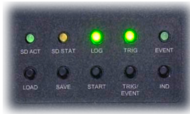
Figure 5. LOG and TRIG LEDs lit
